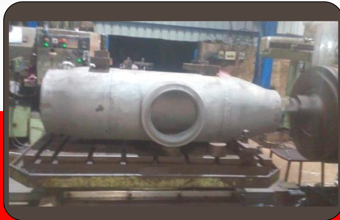
P22 Mixing Tee Spool Client: IOCL
